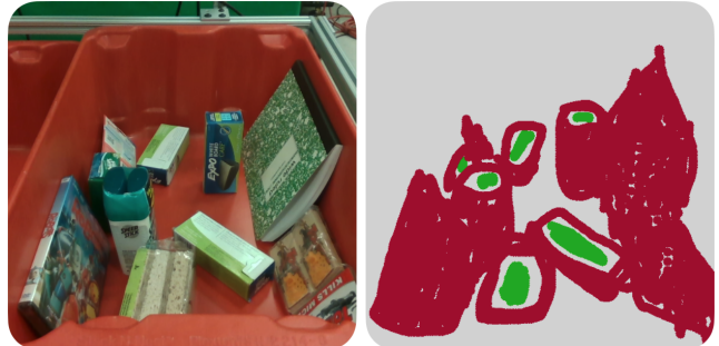
Figure 3: Grasp Affordance Prediction [ARC Grasping; Zeng et al. 2017]. Given objects in cluttered bins, segment the image corresponding to “graspable” (green), vs. “non-graspable” (red) regions; note that these regions are labeled for use with suction grippers .
