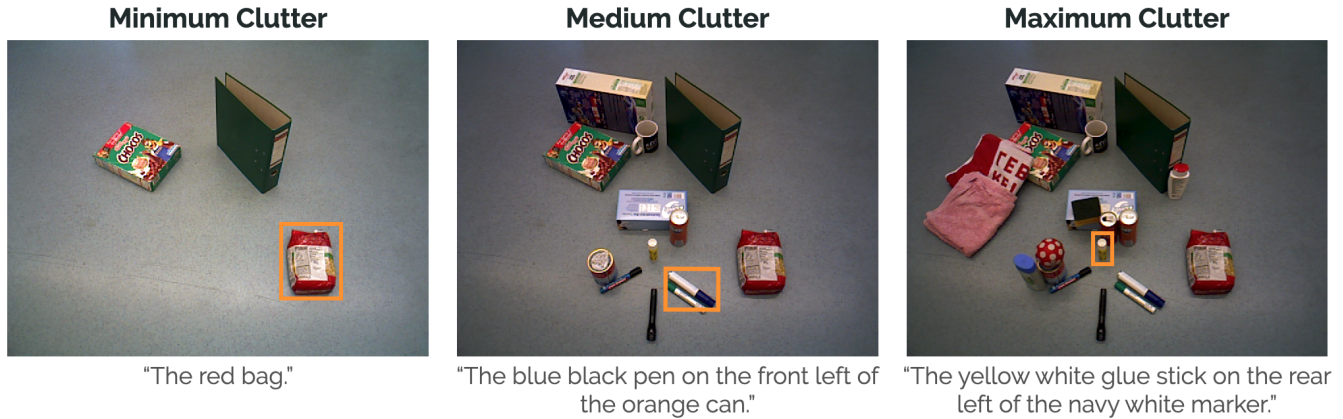
Figure 4: Referring Expression Grounding (Object Detection) from the OCID-Ref Dataset [Wang et al. 2021]. Given a referring expression in natural language, the goal is to predict the bounding box coordinates around the respective object. An important feature of OCID-Ref are the various dataset splits, corresponding to three increasing amounts of clutter, depicted left-to-right.
